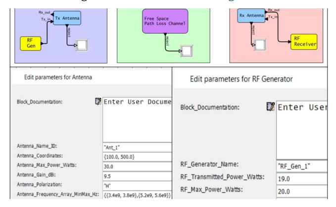
VisualSim Antenna Designer is a datasheet-driven antenna simulation platform for communication system feasibility, evaluate antenna response to real-life scenarios and compare antennas for an application.
